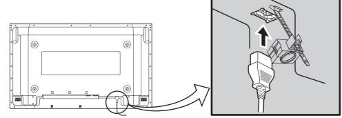
Fix the AC cord plug securely to the Plasma Display with the clamper. (see page 7)
